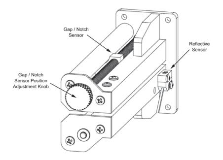
Turn the knob Clockwise to move the sensor toward the outside edge
